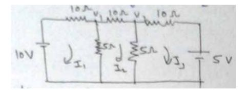
Q5. Write node equations and calculate V1 V2 and V3
